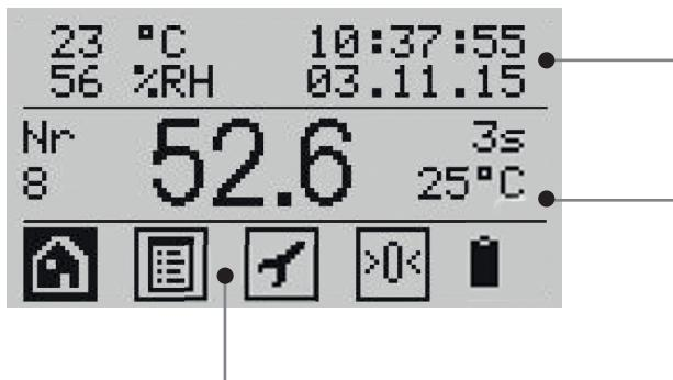
The top section of the display indicates the ambient temperature and humidity, current date and time.
